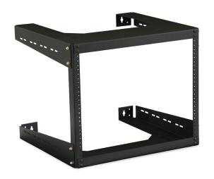
The 0E-WMR8RMS is an 8U hinged wall mount bracket for easy panel installation. Heavy duty steel construction. Supports 125 pounds. 10-32 threaded rack rails. All mounting hardware included. 17.15" H x 19.71" W x 18" D.
